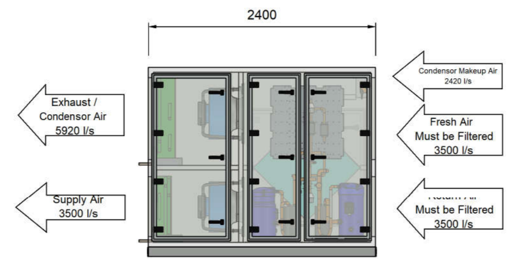
ELEVATION VIEW - COMPRESSOR ACCESS PANEL SIDE
