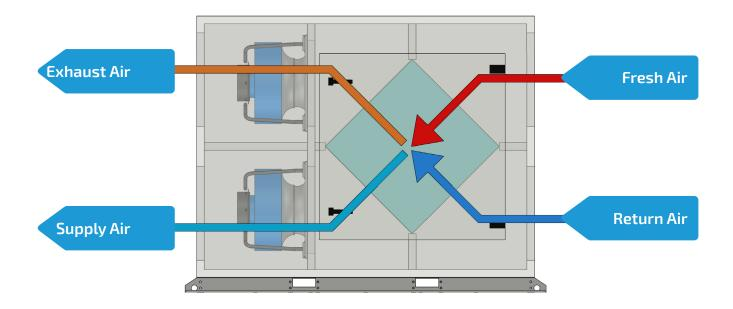
The option shown above does not require any changes to the fan positions inside the unit.
